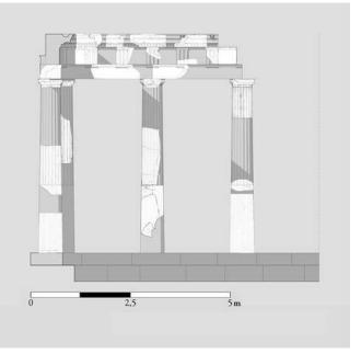
Figure 9: Kos, West Gymnasium. Anastylosis project, east elevation (F. Gotta).
