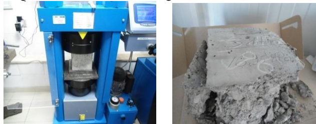
Figure 3.1.1: Compressive strength machine
