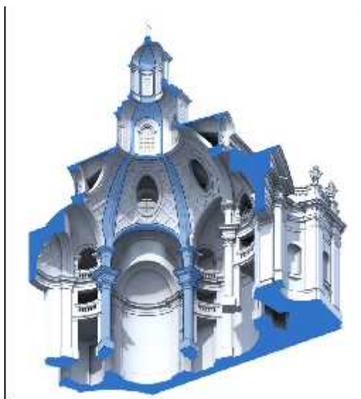
Figure 4 Church of Santa Chiara: continuity of virtually bearing elements
