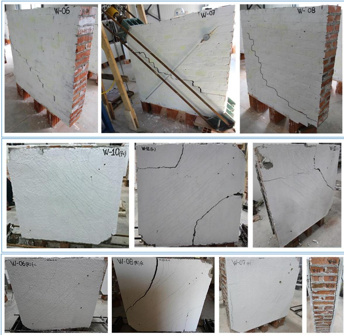
Figure 6. Failure mode of plain, ferrocement strengthened and repaired panels.
