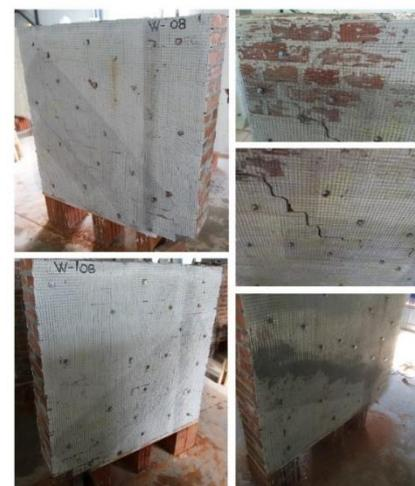
Figure 2. Plastering process with ferrocement jacketing (FC) (schematic view and application) (left) and repairing with ferrocement (right).
