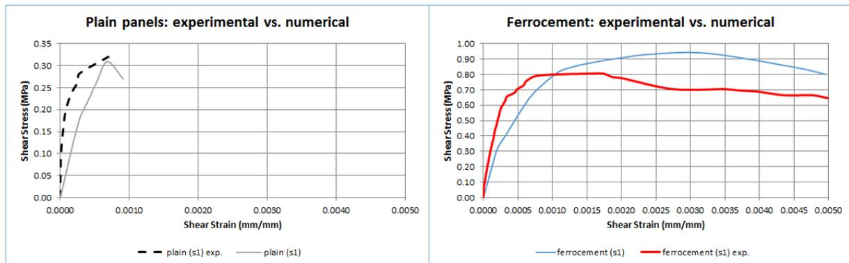
Figure 8. Comparison between experimental and numerical results of plain and ferrocement strengthened panels.
