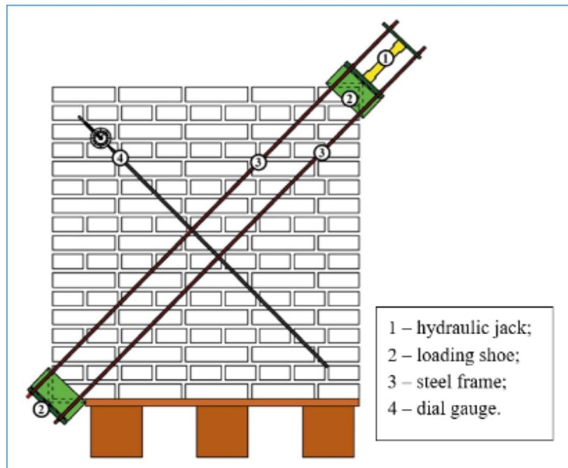
Figure 3. Diagonal compression test set-up.
