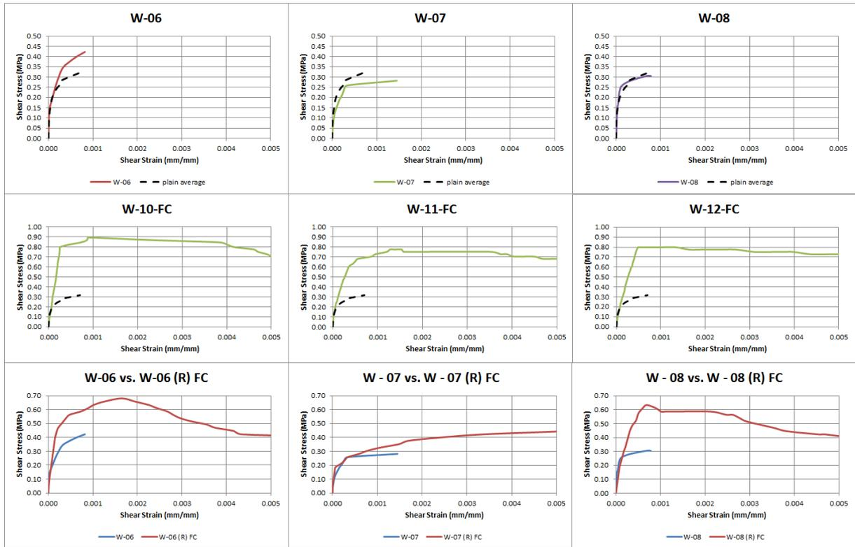
Figure 7. Summary of shear stress vs. shear strain of plain, ferrocement jacketing reinforced and repaired panels.
