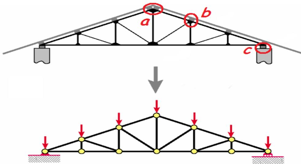
Figure 2 Roof structure and its idealization model
