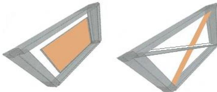
Figure 5 Timbers to braced frame
