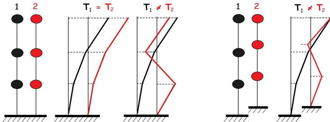
Figure 6 Behavior of buildings with similar or different characteristics
