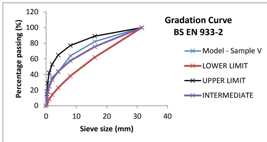
Figure 4 – Gradation Curve Sample V
