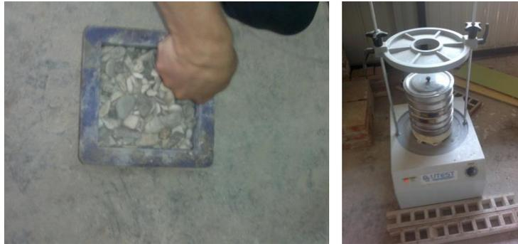
Figure 3- Compaction for rodded unit weight determination; sieve shaking for sieve analysis (starting from the left)
