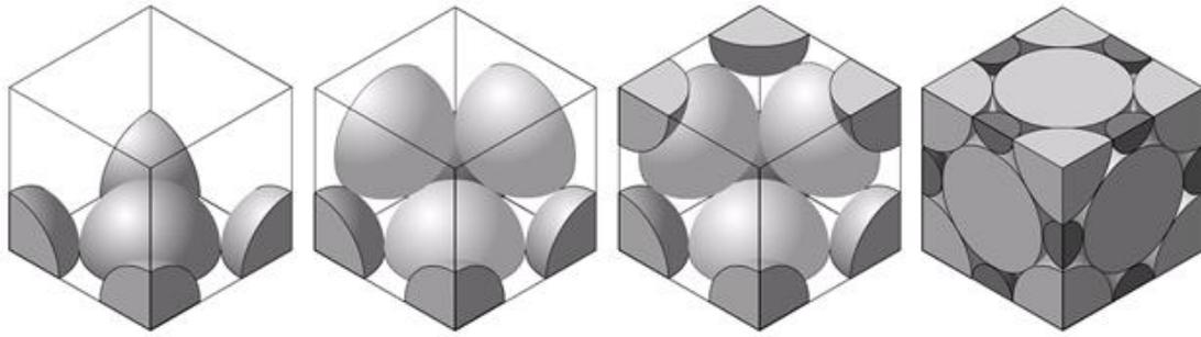
Figure 1-Face Centered Cubic structure when the interstitial spaces are packed with smaller spheres on a unit volume
