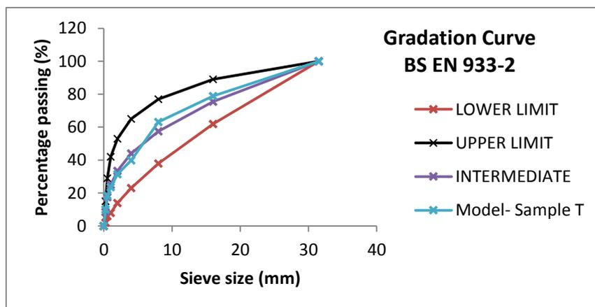
Figure 10 – Gradation Curve Sample T
