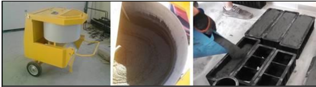
Figure 9 Preparation of test specimens
