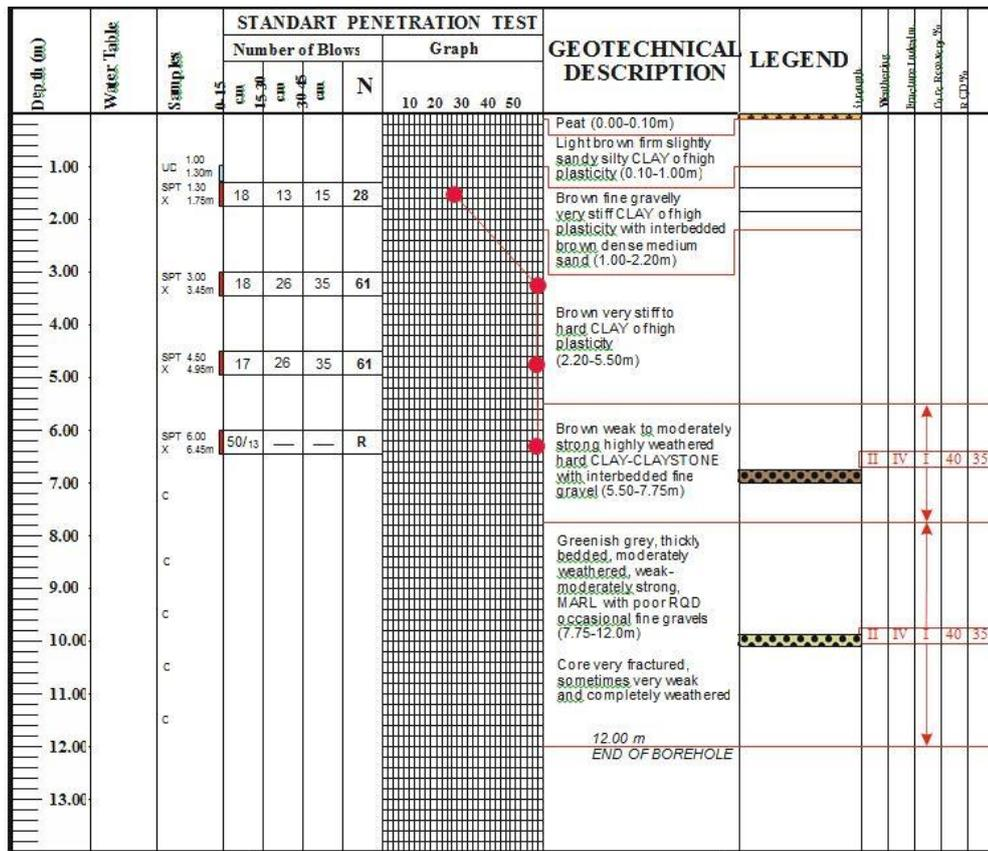
Figure 1 Standard penetration test in Haspolat region
