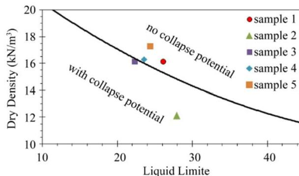
Figure 3 Collapse potential to Liquid Limite and Dry Density
