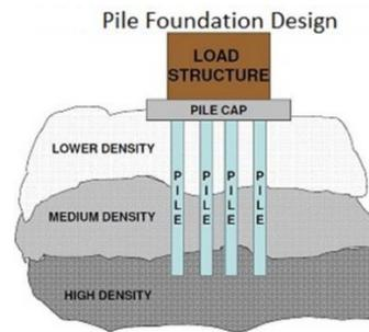
Figure 6 Pile foundation in expansive soils
