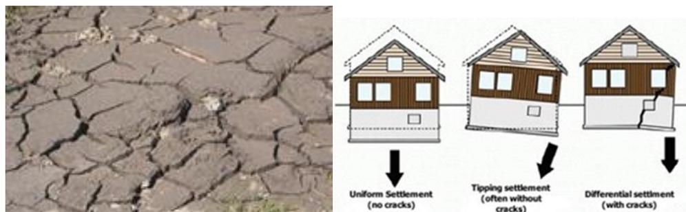
Figure 2 Expansive soil and its effect on buildings
