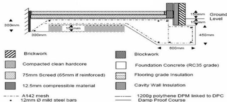
Figure 4 Raft foundation on expansive soil
