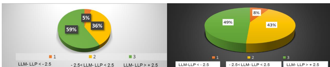
Figure 14. Accuracy in lap length bars according EN and ACI for beams in 7 th floor and for beams in object “Dorado”
