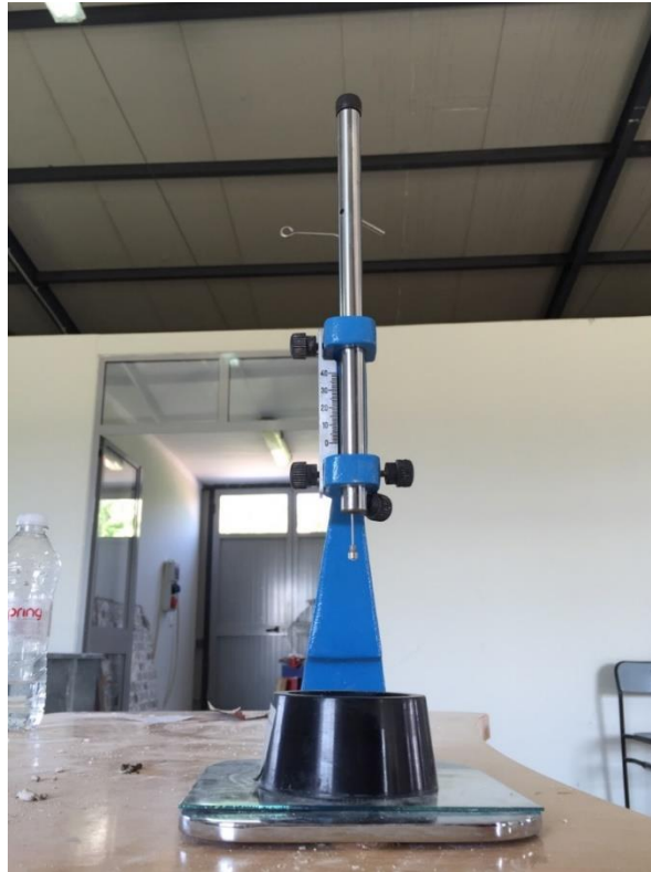
Figure 14. Vicat apparatus finding Normal consistency, initial and final setting time
