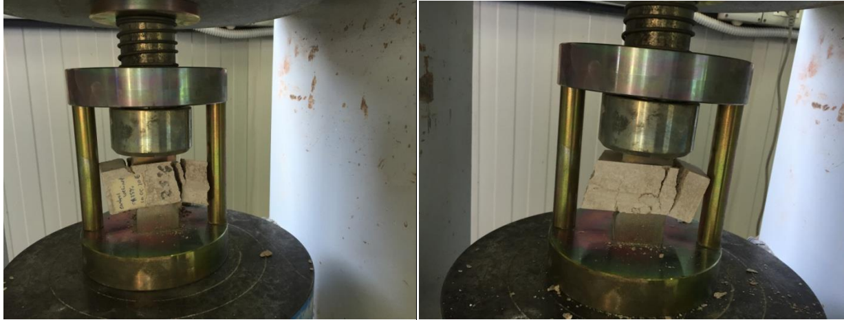
Figure 25. Determination of the Compressive Strength
