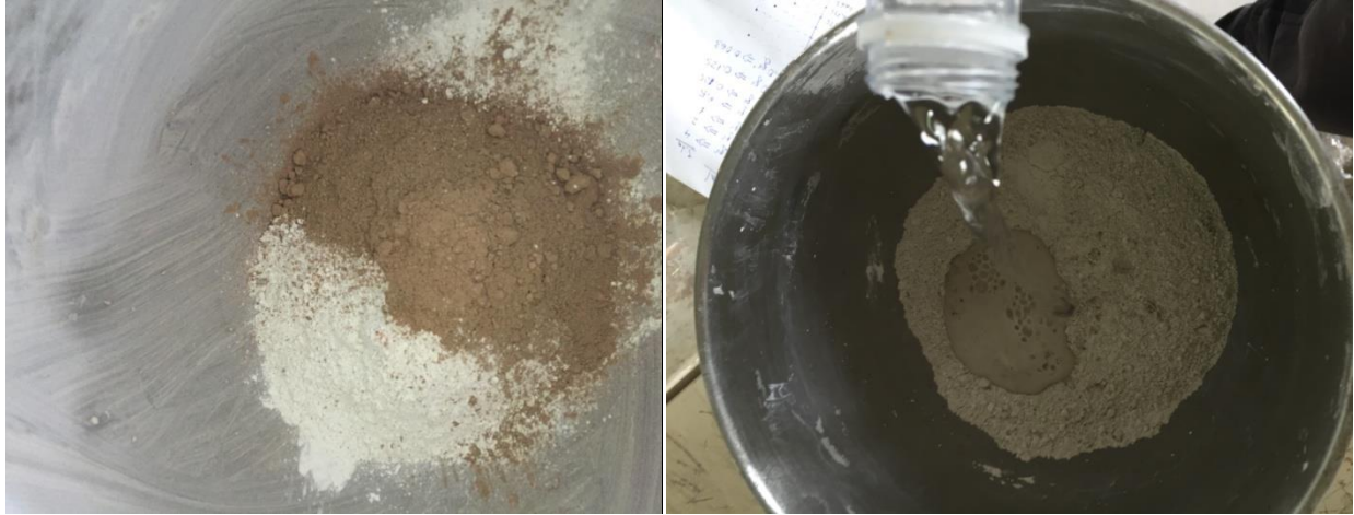
Figure 18. Preparations of the Specimen Mixtures
