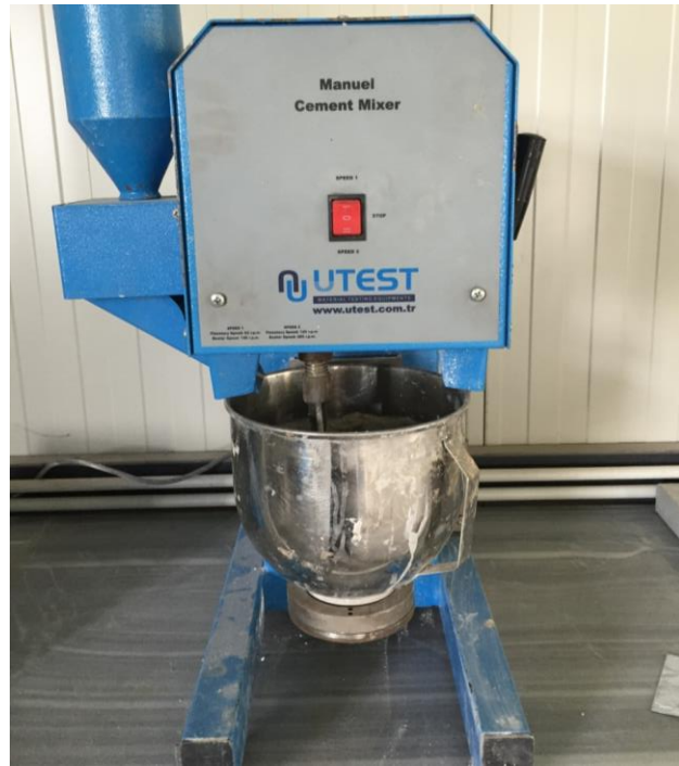
Figure 20. Manual mortar mixers
