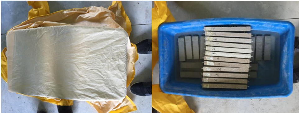
Figure 26. Shrinkage test samples
