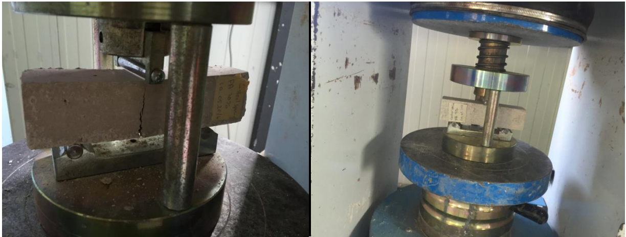
Figure 24. Determination of the Flexural Strength
