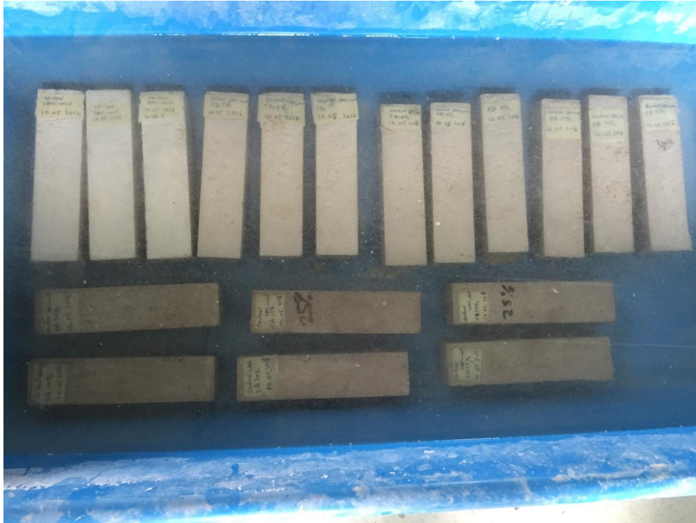
Figure 23. Curing of mortar specimens
