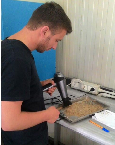
Figure 17. The drying process was dried by hair drying
