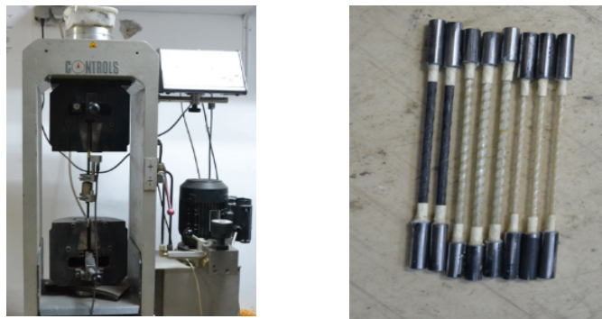
Figure 1. Testing the mechanical properties of Reinforced bars (GFRP CFRP)
