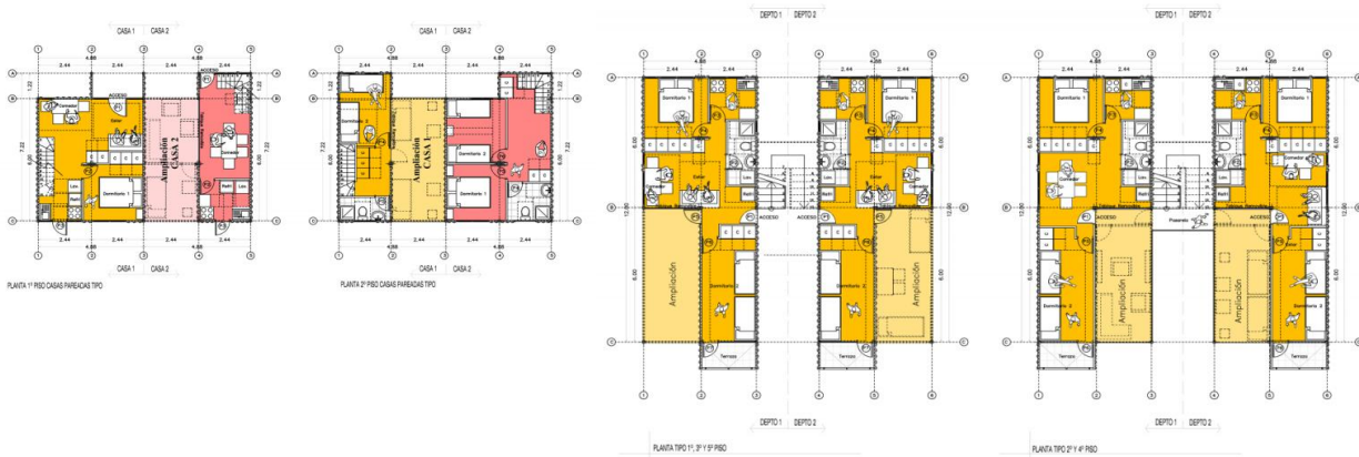
Fig. 5: Container housing: the typical floor plans of 2 story and 5 story buildings.
