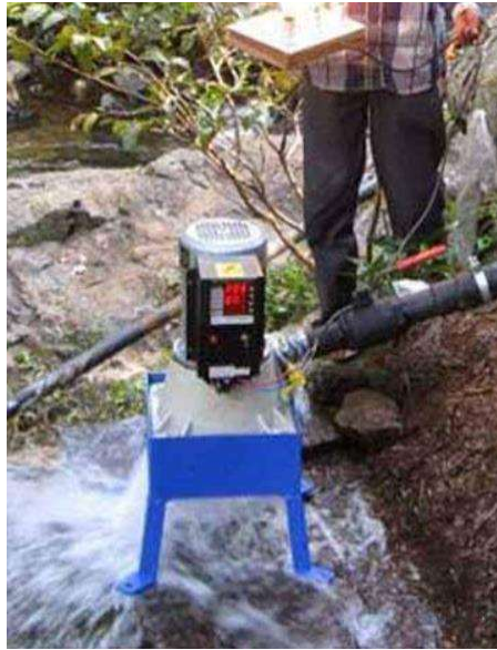
Figure 10: Portable Pico-hydro Power Generation [Paksolarservices].
