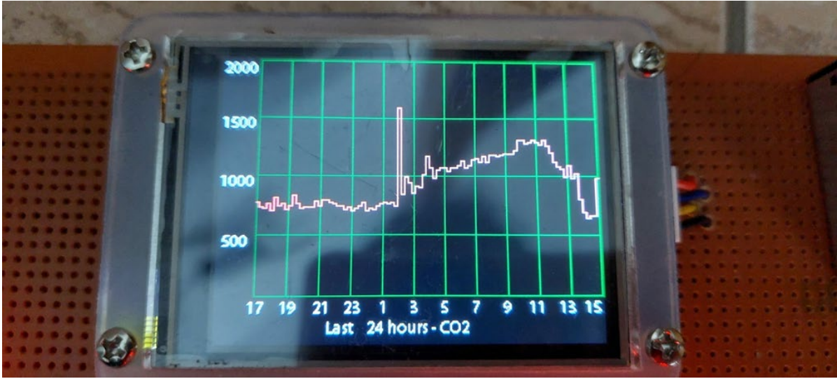
Figure 32. CO2 Graph Representation of 24 Hours Measurement
