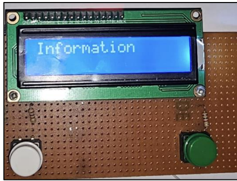
Figure 26. Information menu, if the Ok button (in green) is pressed, information about the health parameters measured by the device is opened.
