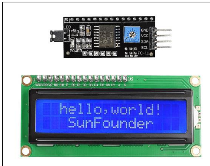
Figure 21. Block sensor diagram 16x2 LCD with I2C communication proto
