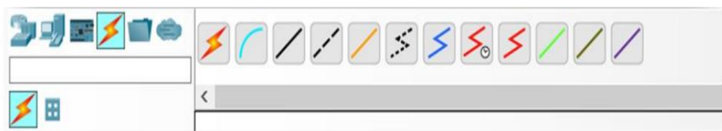
Figure 6. Cables available in the CPT (in the lower left corner we see the auto-cable function)
