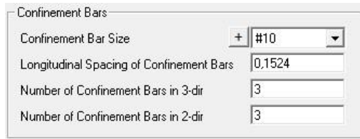
Figure 20. Reinforcement detail for Confinement Bars
