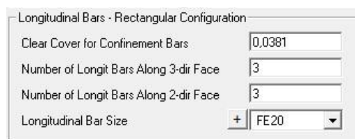
Figure 19. Reinforcement detail for Longitudinal Bars
