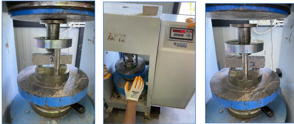
Figure 14 Determination of mortars flexural and compressive strength
