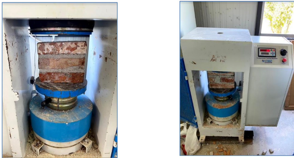
Figure 15 Determination of masonry assemblage compressive strength
