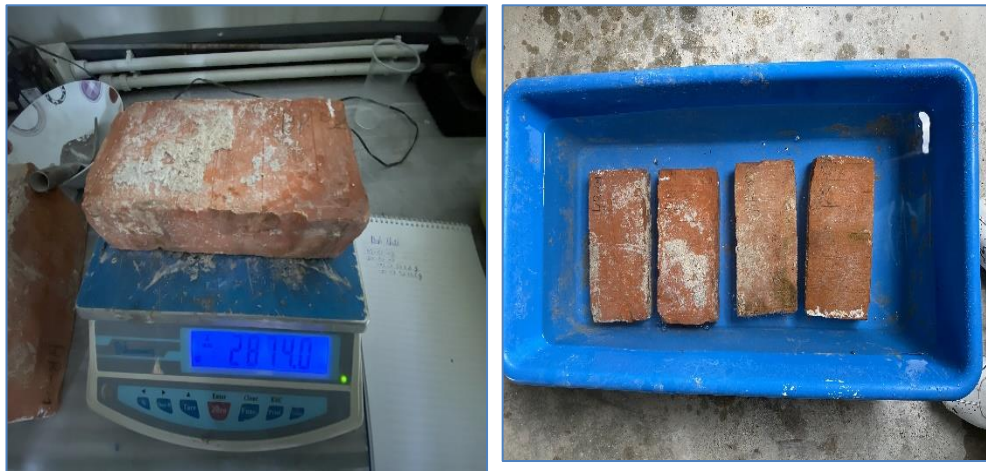
Figure 13 Determination of brick water absorption.
