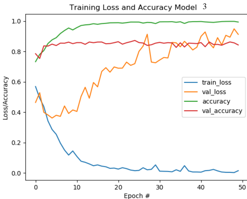
Figure 32. Loss and accuracy for model with LeNet architecture
