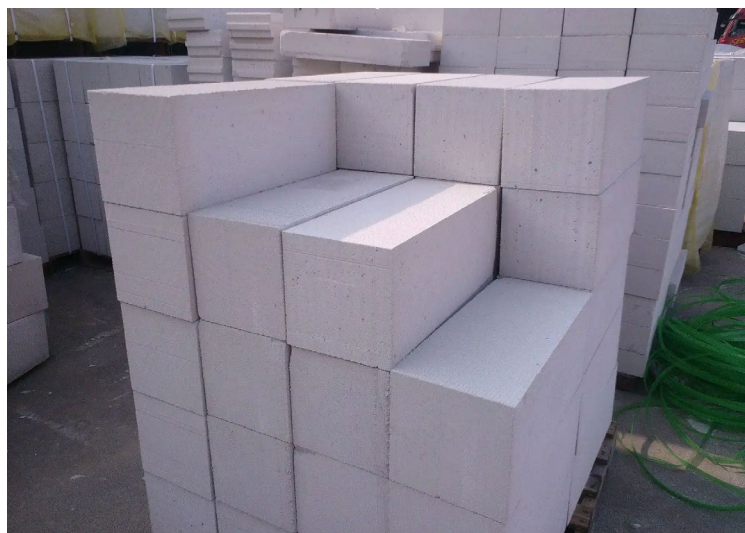
Figure 3. Autoclaved Aerated Concrete (AAC)
