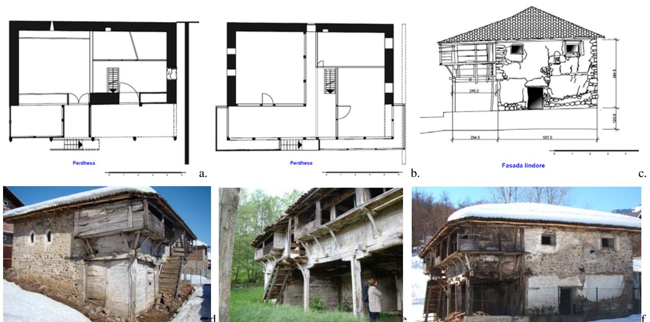
Fig. 1: The dwelling-garret type in Lebusa, Kosovo; a. ground floor layout; b. first floor layout, c. east elevation; d. west-south view; e. south view; and f. east view.
