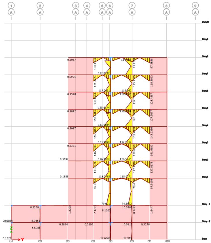
Figure 58 Moment 3-3 for internal frame A
