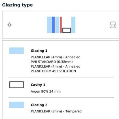
Figure 26. Double Glazing configuration DG_5.2.
