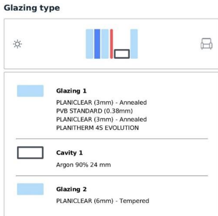
Figure 14. Double Glazing configuration DG_1.2.
