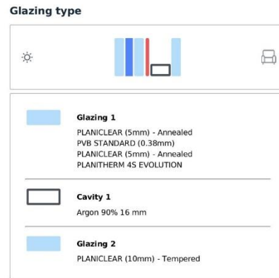
Figure 33. Double Glazing configuration DG_8.
