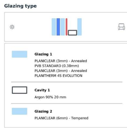
Figure 13. Double Glazing configuration DG_1.1.
