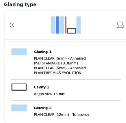
Figure 39. Double Glazing configuration DG_10.
