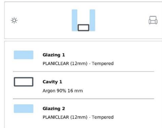
Figure 119. Double Glazing conceptual section drawing (configuration) of glazing scenario DG_9, (Air Albania Stadium case).
