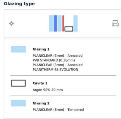
Figure 19. Double Glazing configuration DG_3.1.
