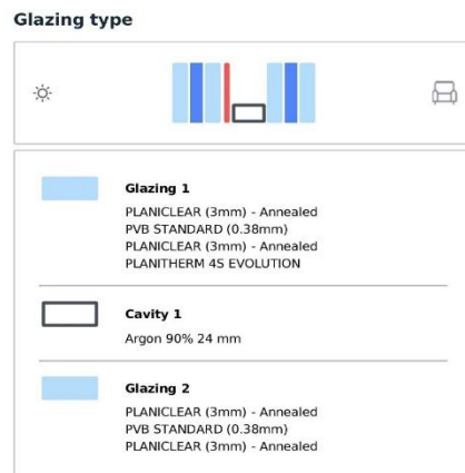
Figure 17. Double Glazing configuration DG_2.2.
