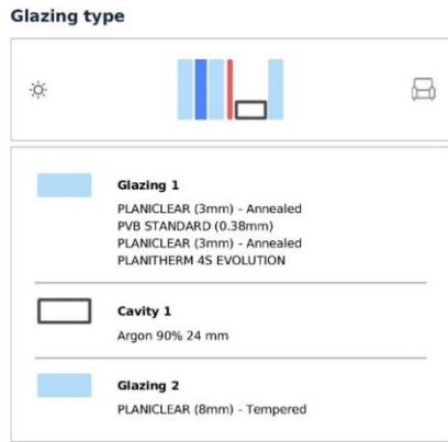
Figure 20. Double Glazing configuration DG_3.2.
