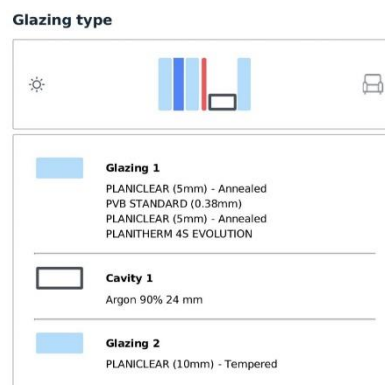
Figure 35. Double Glazing configuration DG_8.2.
