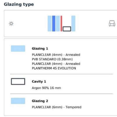
Figure 21. Double Glazing configuration DG_4.
