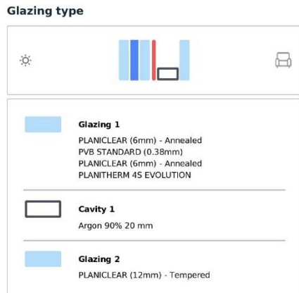
Figure 40. Double Glazing configuration DG_10.1.
