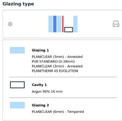
Figure 12. Double Glazing configuration DG_1.
