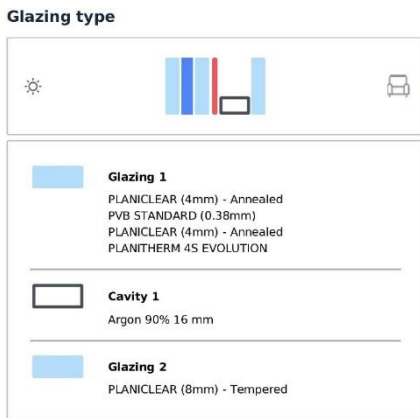
Figure 24. Double Glazing configuration DG_5.
