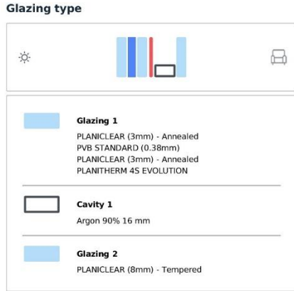
Figure 18. Double Glazing configuration DG_3.
