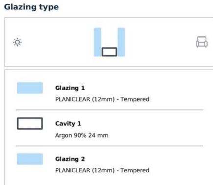
Figure 38. Double Glazing configuration DG_9.2.
