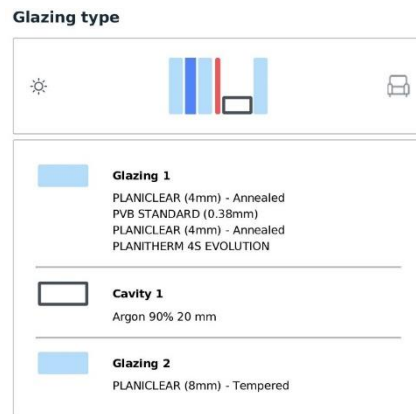
Figure 25. Double Glazing configuration DG_5.1.
