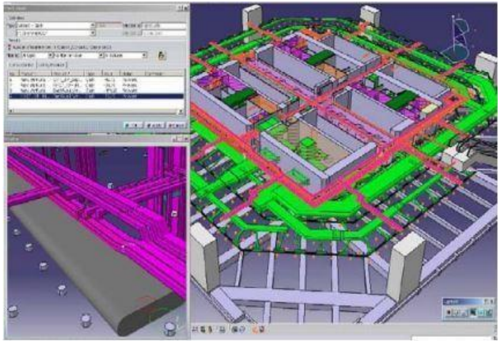
Figure 14: Automated clash detections
