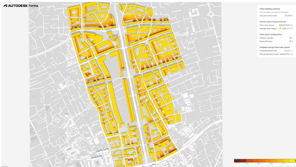
Figure 57 Solar Energy Potential
