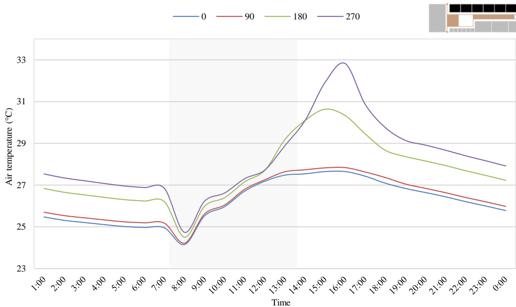
Figure 93. Simulated indoor air temperatures of classrooms of BL typology in terms of rotation angle for 12th of September
