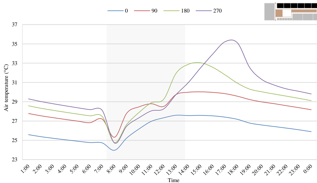
Figure 96. Simulated indoor air temperatures of classrooms of BL typology in terms of rotation angle for 12th of September
