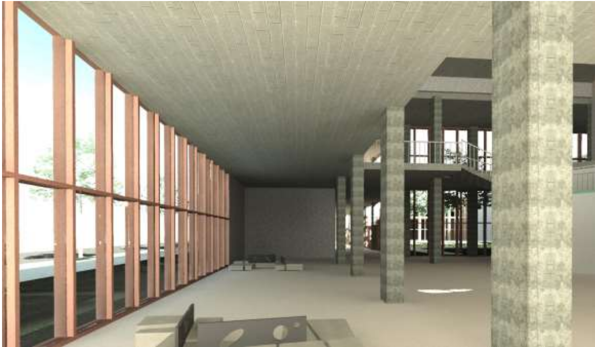
Figure 81. Interior Details of construction materials. Bronze Structural glazing combined with cast in place concrete create a modern setting
