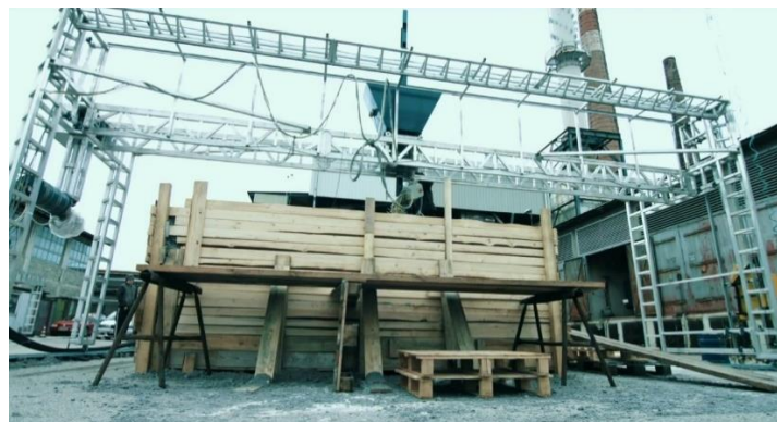
Figure 11. BetAbram P1 3D Printer, image source www.youtube.com
