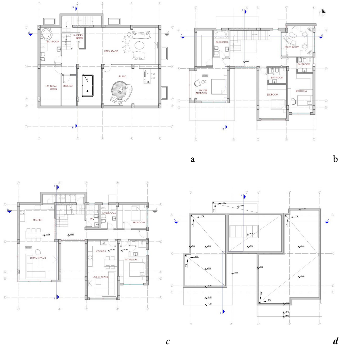
Figure 31. a. Underground floor plan, b. First- floor plan, c. Second floorplan, d. Terrace floor plan (Cani, 2023 )
