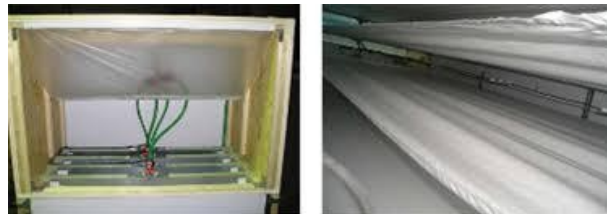
Figure 6. 'Experimental setup-top of the tower (left) and textiles used as moist surfaces (right) (F. Babich, M. Cook, J. Cremers, G.Papachristou, 2017)
