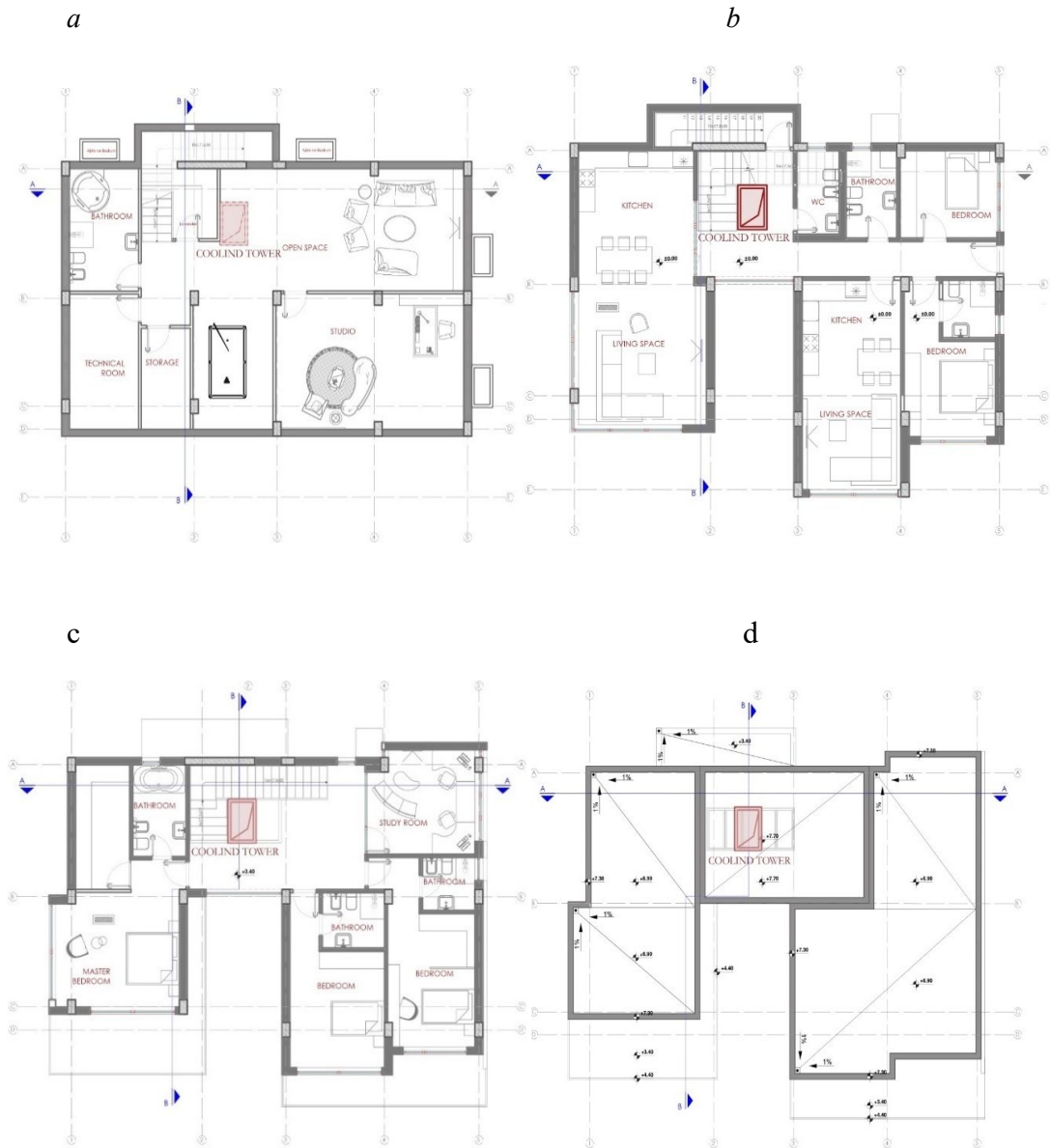
Figure 36. a. Underground floor plan, b. First- floor plan, c. Second floor plan, d. Terrace floor plan (Cani, 2023)
