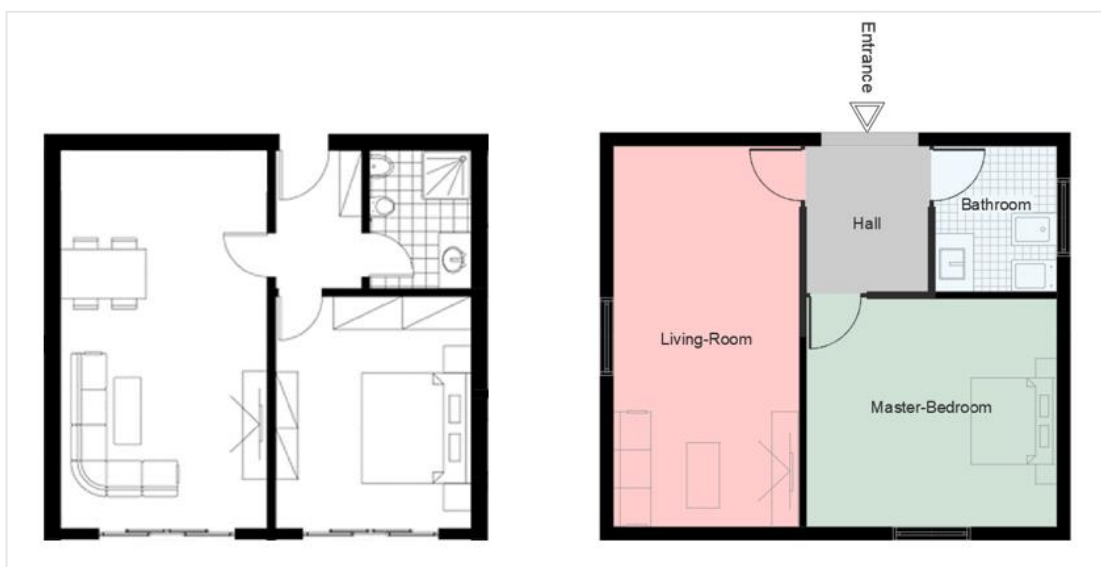
Figure 51: Analysis for calibration purposes. The original plan (on the left), the twin generated plan (on the right)
