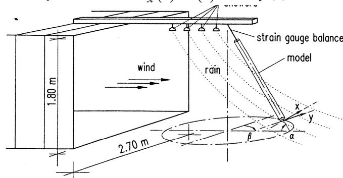
Fig.1 Wind tunnel test (inclination and deviation angle)
