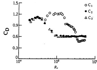
Fig.9 Drag coefficient-Reynolds number relation  $C_1 - C_3$
