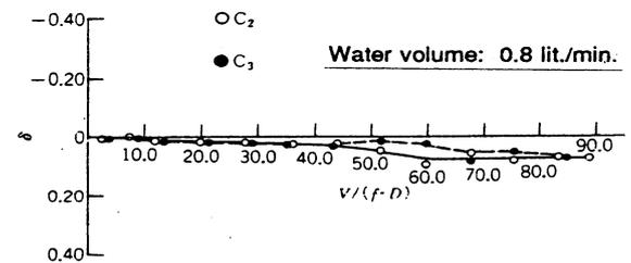
Fig.12 Damping characteristics for the model C<sub>2</sub> and C<sub>3</sub>
