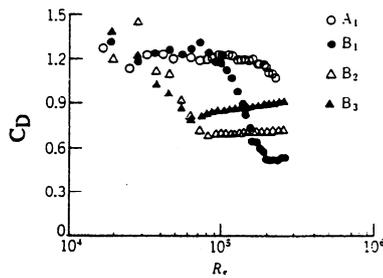
Fig.8 Drag coefficient-Reynolds Number relation  $B_1 - B_3$
