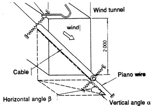
Fig.10 Model fixation
