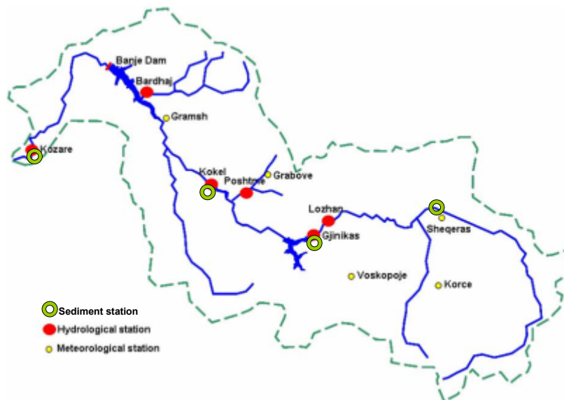
Figure 4.2-1. Map of River Devoll with stations for hydrology and meteorology and water sampling for suspended sediment analyses (labelled “sediment station”).
