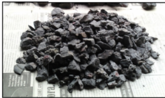
Figure 4. FCS specimen for Los Angeles abrasion test
