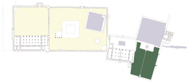
Figure 2: Lal Mahal. Ground level plan showing the aggregation of the two western compounds and the rotated eastern pavilion adjacent to the garden area and the second water tank which a domed structure has been built by its eastern side. Architectural survey by the author and Fabrizia Dragone (February 2014)
