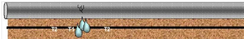
Figure 5: The detection of the water leakage with the help of the cables, laid below the pipeline (Inaudi and Glisic, 2006)
