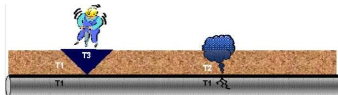
Figure 6: The detection of the gas leakage with the help of the cables, laid above the pipeline (Inaudi and Glisic, 2006)
