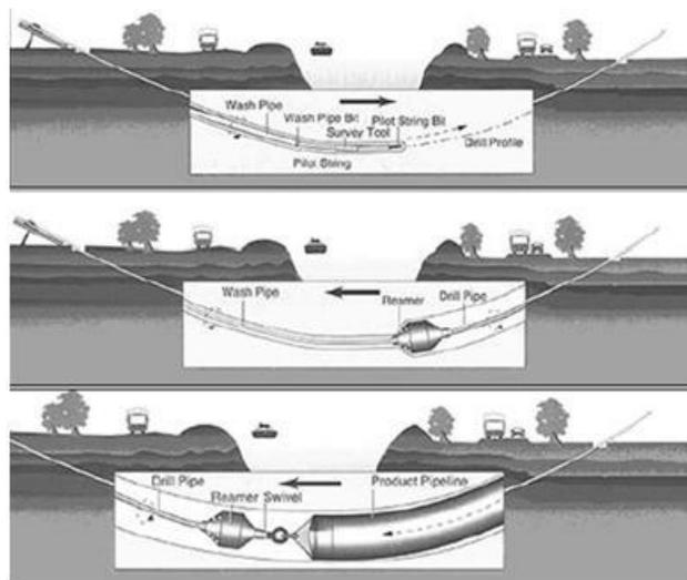
Figure 2: Stages of Horizontal Directional Drilling (Opening of the guide hole, expanding the hole and pulling the Pipe) (Willoughby, 2005)
