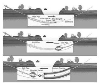
Figure 2: Stages of Horizontal Directional Drilling (Opening of the guide hole, expanding the hole and pulling the Pipe) (Willoughby, 2005)
