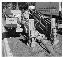
Figure 1: Horizontal Directional Drilling Equipment (Willoughby, 2005)
